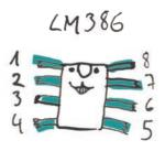
Amplifier Chip: This is named LM386, and looks like an insect with a little notch on its head. The leg at the left side of the notch-head is leg number one. Count counter clock wise from leg number one and give each leg a different number.
